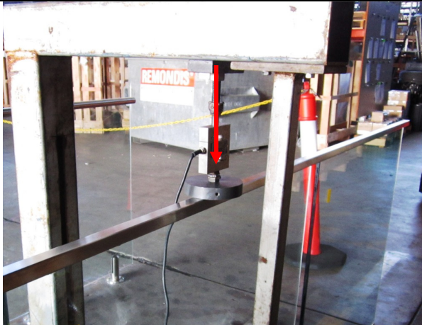
Photo 5 Hand Rail Loading Downwards
