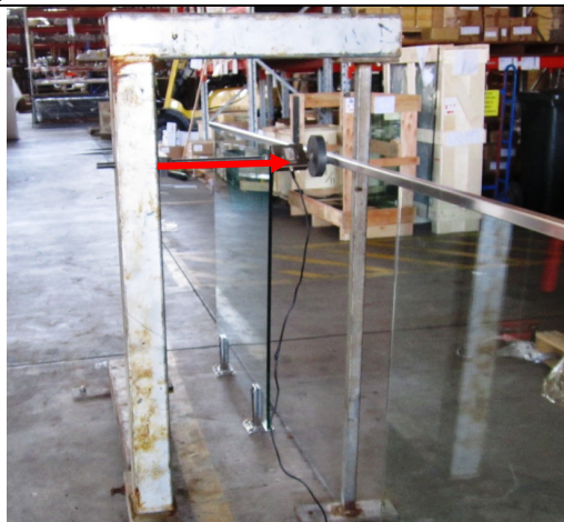
Photo 6 Hand Rail Loading Outwards with middle panel removed - AS 1288
