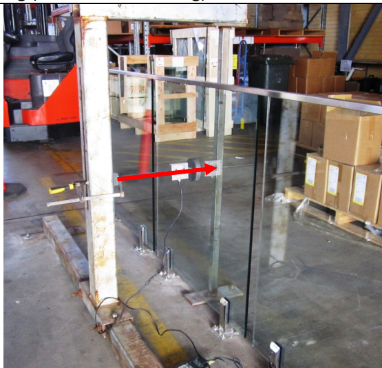
Photo 9 Any Direction (Point Loading)(Arrow represents actual load location & direction)
