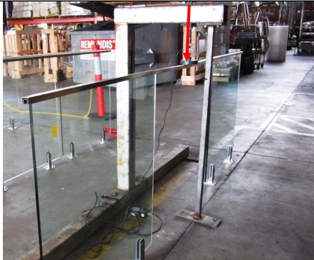
Photo 7 Hand Rail Loading Downwards with middle panel removed – AS 1288
